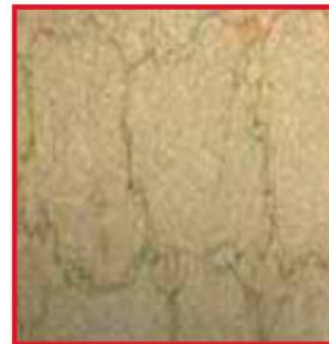
Typical silicate discolouration on the surface of the instrument after steam sterilization caused by excessive silicon dioxide levels in the demineralised water
