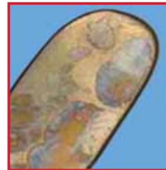
Typical silicate discolouration on the surface of the instrument after steam sterilization caused by excessive silicon dioxide levels in the demineralised water
